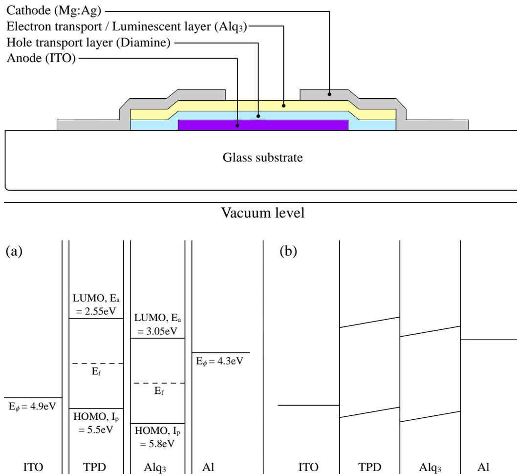
**Figure 1.2-1: Schematic of first modern OLED and energy levels**
