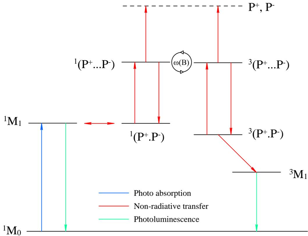
**Figure 1.4-1: Frankevich schematic for magnetic modulation of photocurrent**
