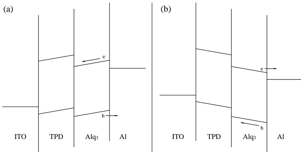
**Figure 3.3-9: Schematic of band structure around  $V_{oc}$  for an Alq<sub>3</sub> OLED**
