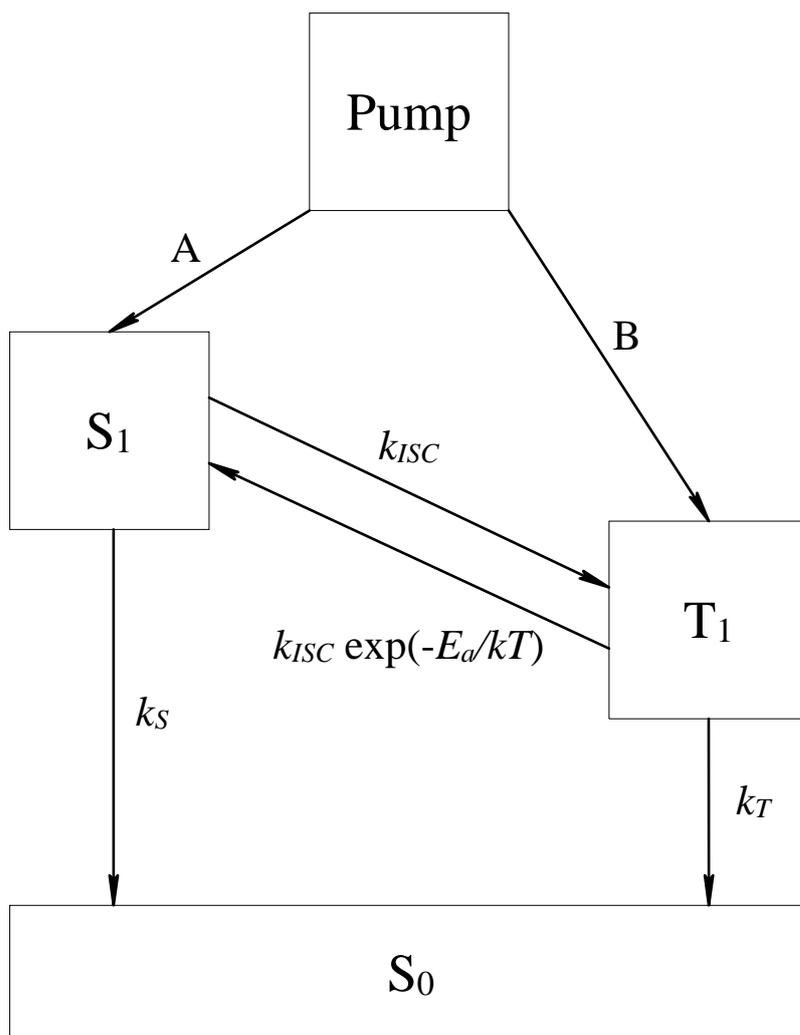
**Figure 3.2-8: Rate schematic between exciton states in Alq<sub>3</sub>**
