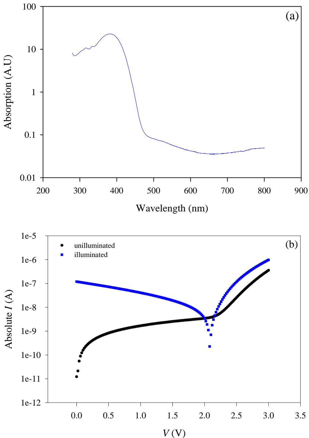
**Figure 3.3-1: Absorption spectra of Alq<sub>3</sub> and IV curves for an OLED with and without illumination**
