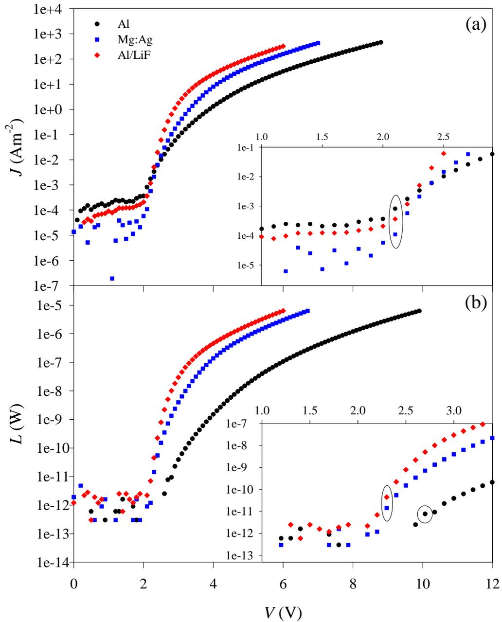
**Figure 3.1-1: V against J and V against L curves for Alq<sub>3</sub> OLEDs with various cathodes**
