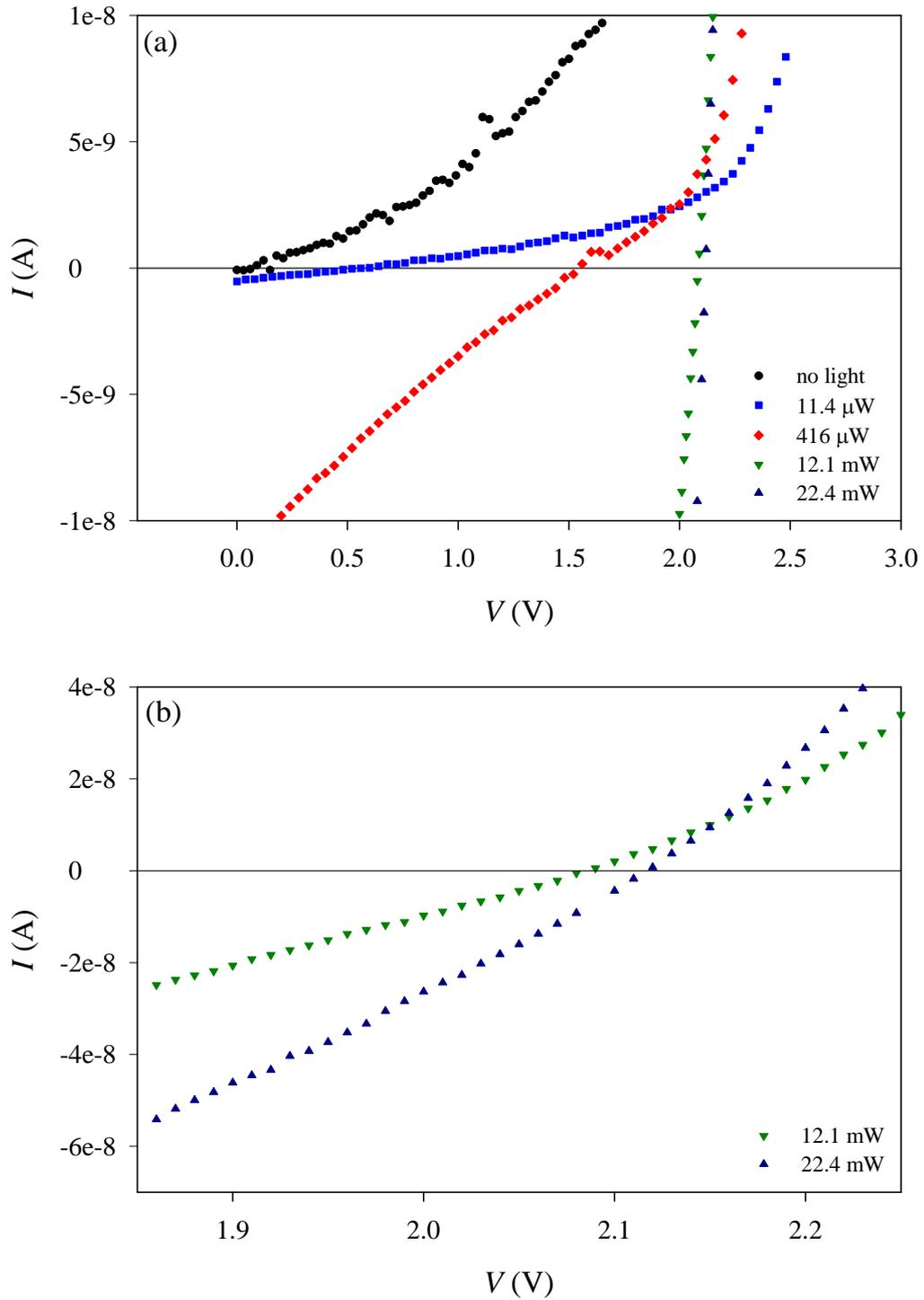
**Figure 3.3-5: *I**V* of Alq<sub>3</sub> OLED with various levels of illumination**
