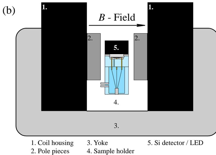
**Figure 2.2-1: OLED sample holder and magnetic measurement schematics**
