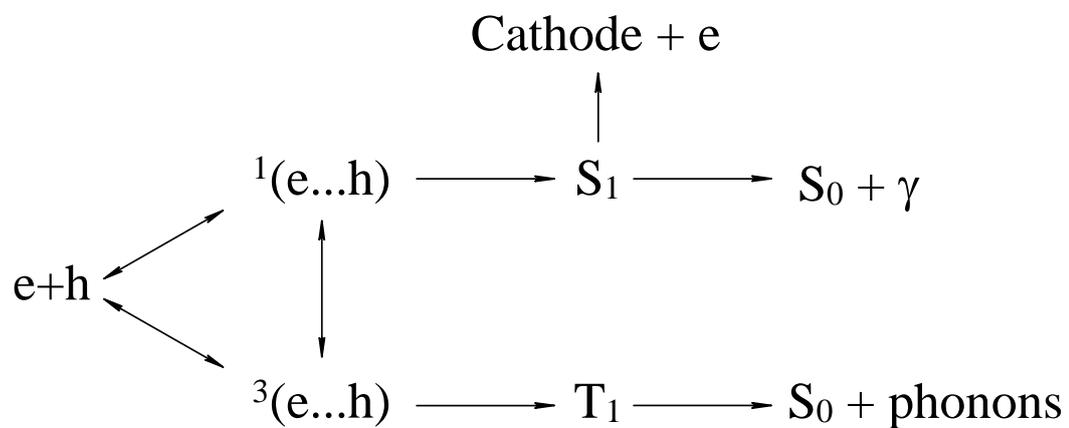
**Figure 1.4-3: Kalinowski rate schematic for an Alq<sub>3</sub> OLED**
