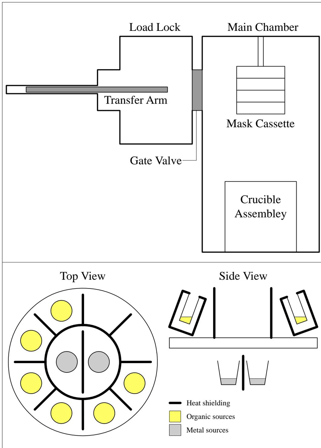
**Figure 2.1-2: OLED growth system schematic**
